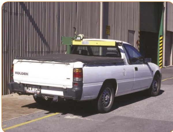
F12643 Backsaver Crane mounted on Holden Utility vehicle
